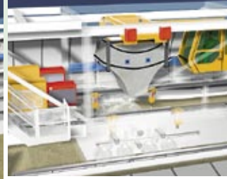
④ The prefabricated concrete elements are transported to the tunnel boring machine through the backup system ...
