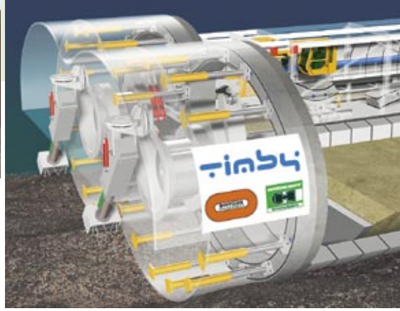
③ Two cutting mill arms cut the lower tunnel contour into the riverbed.
